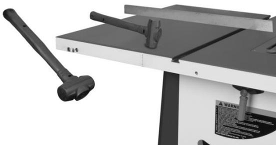
Figure 5-5: leveling extension wings, method
