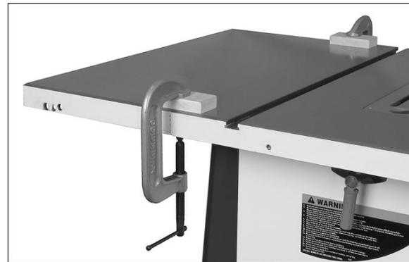
Figure 5-6: leveling extension wings, method 2
